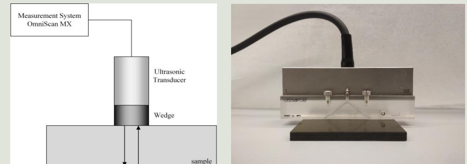
Figure 4. Experimental set-up for the inspection with phased array.
