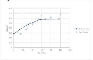
**Overprediction** of  $G_c$  for short crack extensions VS **Underprediction** of  $G_c$  for longer crack extensions
