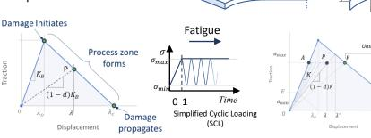
The CZM is implemented in a UMAT in Abaqus for FE analysis
